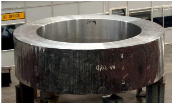
750 mm thick Ring Forging for Flange Area of RPV-OD5300 x ID3800 x 700L
